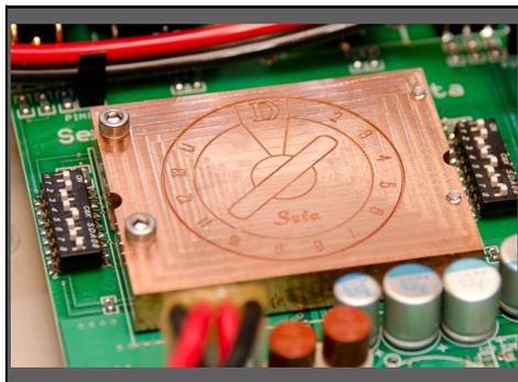
**The Seta DAC Buffer uses a unique video - bandwidth amplifier module which is electronically and acoustically isolated as well as kept at a stable operating temperature and environment (constant humidity) by enclosing and sealing in a block machined from a solid piece of oxygen-free high conductivity copper.**
